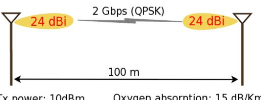
Tx power: 10dBm Bandwidth: 1.5 GHz SNR: 15 dB Oxygen absorption: 15 dB/Km Noise figure: 6 dB Link margin: 10 dB 100-200m very doable Kilometers range is overreach even without oxygen absorption (rain loss as high as 30 dB/km)
