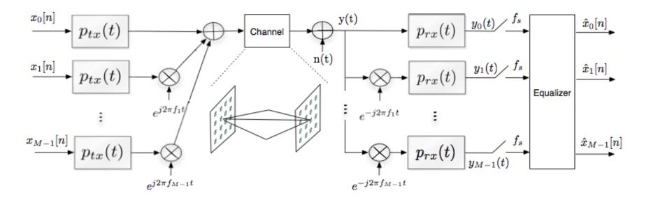
How to scale communication bandwidth? --without ADC advances? --still leveraging Moore's law Sloppy analog channelization, "slow" ADCs and DSP in parallel
