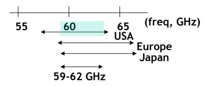
Oxygen absorption band Ideal for short-haul multihop (reduced interference)
